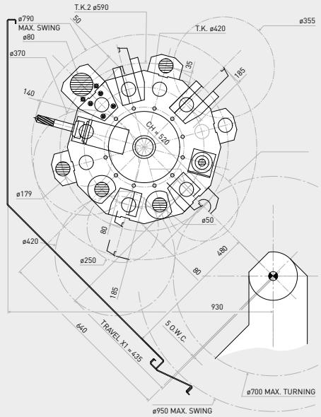
**Right spindle 80 version (V6) with standard turretMASTER**
